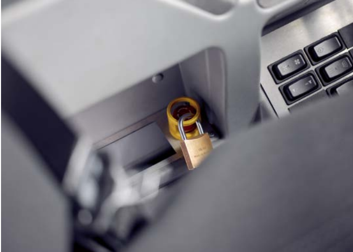
Figure 4 Example of safeguarding against reconnection
