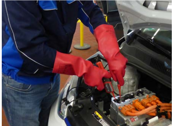
Figure. 5 Verification of the non-live state
