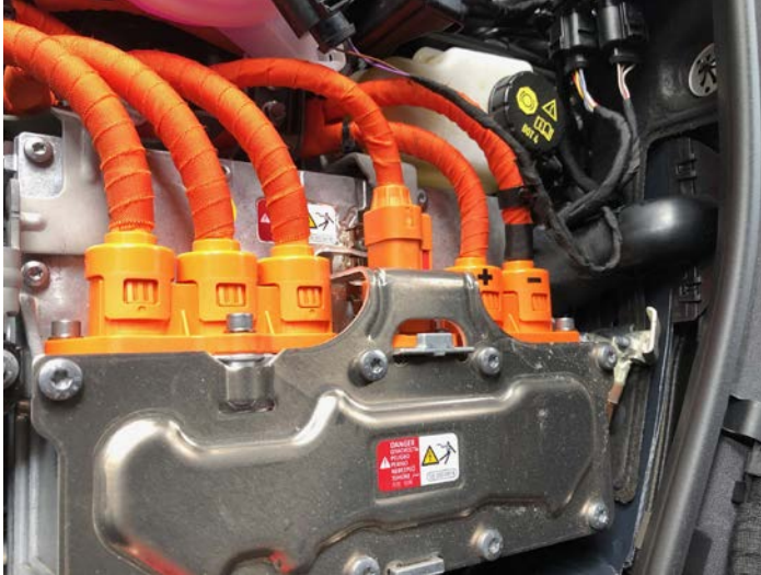
Figure 2 Basic protection by insulation and shrouding
